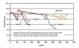
Samples 1 and 2 were charged at 14.2V while Samples 3 and 4 were charged at 14.7V. All batteries were discharged at 2.3A until the terminal voltage dropped to 10.02V and charged for 16 hours. In this particular test, a capacity of 11.5Ah corresponds to 100% capacity and 9.2Ah is 80% of rated capacity and the battery is considered to have reached end of life at that point.
