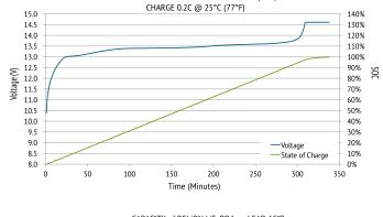
CHARGE VOLTAGE and STATE OF CHARGE (SOC)
