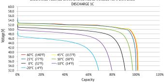
DISCHARGE VOLTAGE CHARACTERISTICS at VARIOUS TEMPERATURES
