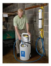
Deionizer system being used to fill Hydrofill watering cart.
